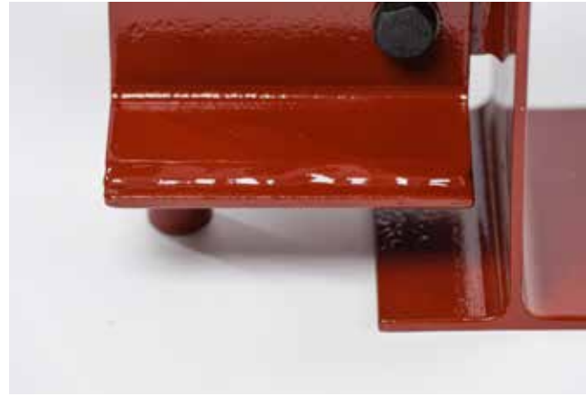
▲ AESS 1: Continuous weld appearance.
